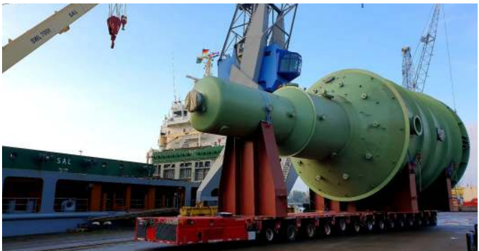
PRE-ASSEMBLED CRYSTALLISERS · BARGE LOADING
